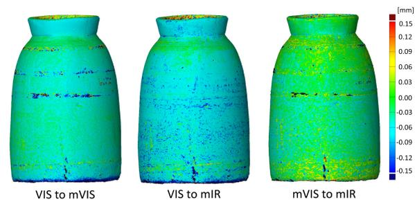
Figure 11. Surface discrepancy maps comparing the three resulting 3D reconstructions of the mango wood vase: VIS to mVIS, VIS to mIR, and mVIS to mIR.
